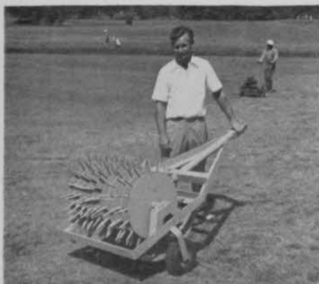
Upside-down view of Bill Perry's homemade Deep Spiker shows construction and wheel attachment.
