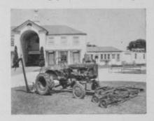
An additional feature is a hydraulic lift device which enables the operator to raise or lower the entire assembly automatically from his normal riding position. With cutting equipment raised entirely free of the ground, the tractor can be moved rapidly from one mowing job to another, across walks, etc.
