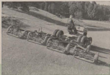
**FOR ECONOMY**—HITCH IT TO THE CHIEF. Particularly designed for work with mowing units, the Chief, with its low fuel consumption and trouble-free performance, hauls this Fairway Mower at top efficiency. With a wheel base of only 68¼", the Chief can turn on an inside radius of 5½ feet . . . a big advantage when working in confined areas.
