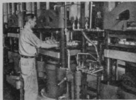
Several hydraulic presses like the above mold and vulcanize the cup-shaped covers on the rubber thread-wound ball. Similar presses produce the required center rubber ball which is the "beginning" of the MacGregor golf ball.
