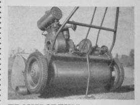
TRANSPORTING. No other mower gives you this simple powered transporting device. Just slide the rubber-tired wheels onto the drive axle, push the clips and head for the next green. You bet it saves time ... and effort too! It's yours at no extra cost.
