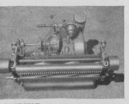
COMBING. Remove nap from greens aily while you cut. An easily attached omb or brush will reach down and lift ach creeper so that it's clipped at the orrect height. This Toro improvement eeps greens in the finest possible condition!
