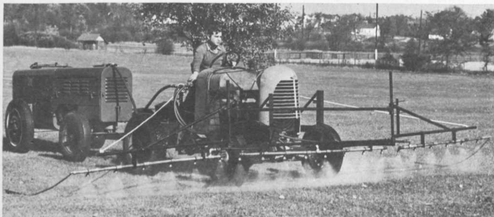
This 20-nozzle boom mounted on the front of a tractor with spray tank towed, makes an efficient rig for 2,4-D application. Flat fan spray and minimum of fog in application. Boom wings are hinged for ease in keeping 2,4-D away from areas where material should not be applied.
