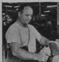
REGGIE McNAMARA , who plays in the low 80's, is a 22-year man with Spalding. Here he is turning the necks of wood club heads.
