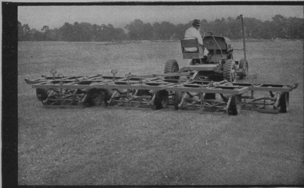
Fast straightaway mowing of your rough with absolute maintenance of height desired. No rollers—grass stands straight after mowing.
