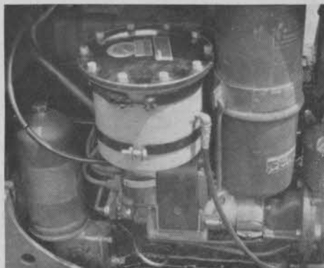
New Fram filter is shown (center) installed on McCormick Deering 1935 model tractor. To the left of filter is old screw type filter no longer used; to right, the oil bath air cleaner.
