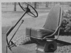
Here's a real comfortable fully upholstered bus seat mounted on a coil spring for easy riding.
