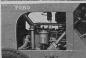
The new Ford Army Scout Car Tractor Engine — Four speed transmission, Clark heavy-duty rear axle, 69½ inch wheel-base, 5.50 x 16 front, 7.50 x 18 rear tires.
