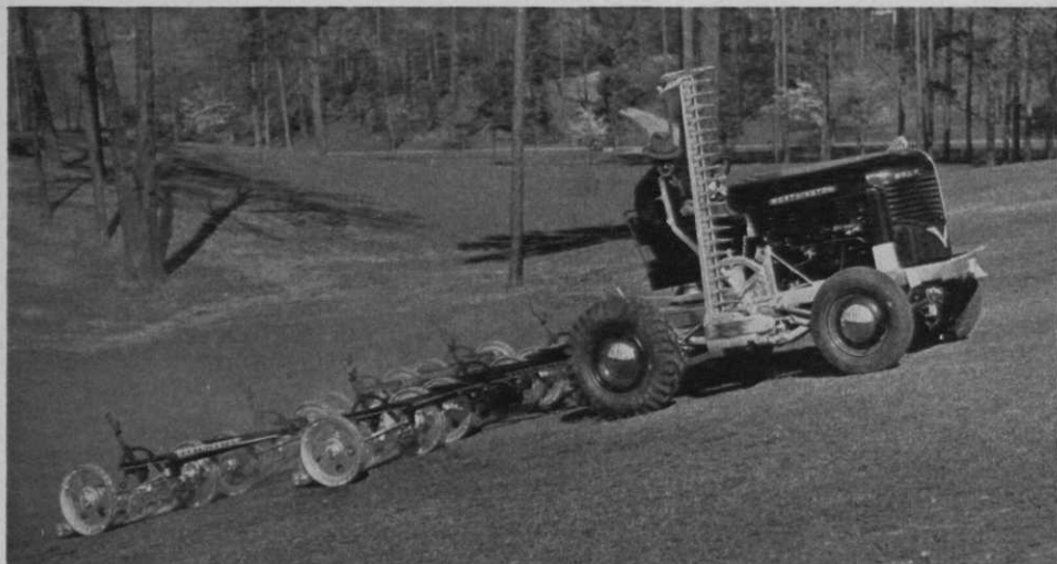
Worthington Golf Chief and 7-Gang Mower at Druid Hills Golf Club, Atlanta, Ga., pulling up steep grade without slippage and without necessity for dual rear wheels.
