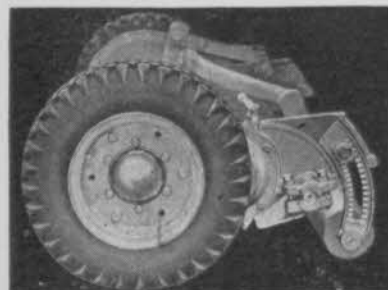
Graduated notched roller brackets. 2\frac{1}{2} inch cutting range . . . a great rough cutter.
