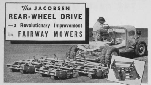
The rear wheel driving power, exclusive in the Jacobsen Fairway Mower, removes any tendency to lift in tough cutting or at high speeds. Hugs the ground like a snake, giving a clean, even cut, and getting dandelions and buckthorn.
