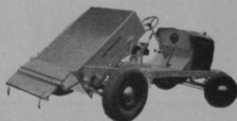
For those who prefer a rectangular type dump body with automatically opening and closing tailgate, the model, illustrated here is recommended.
