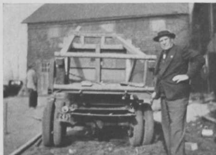
1. Tree mover in position on dump truck which is driven to the tree which Flood has decided to relocate
