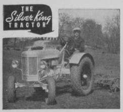
The Silver King is an ideal Golf Course Tractor designed to take care of every service required for complete turf maintenance. Features include: low first cost, unusual economy of op-eration, high speed, ample power, low pressure tires or wide roller type wheels as desired, light weight, four speed transmission, 2½ to 25 miles per hour, Catalog and prices upon request.
