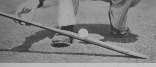
Here's the Stimp meter, which measures the putting speed of turf.
