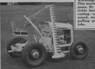
Worthington Sickle Bar Tractor. This tractor is useful for all purposes. By pushing the lever, the sickle bar is lowered ready for cutting—a slight pull and it is raised, readying the tractor for pulling gang mowers and other iobs.
