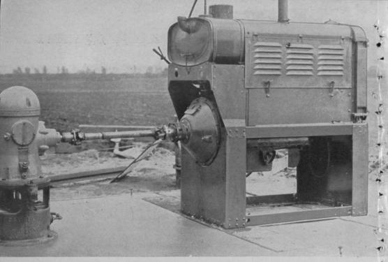
The International Diesel Power Unit operating a pump, providing low-cost pumping power for the owner.
