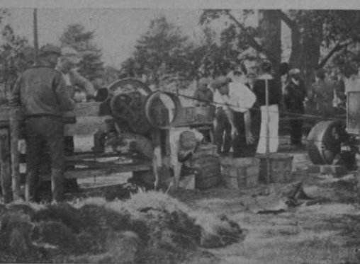
An ensilage cutter prepares the stolons for planting. Tussocks as they come from the nursery are in foreground.
