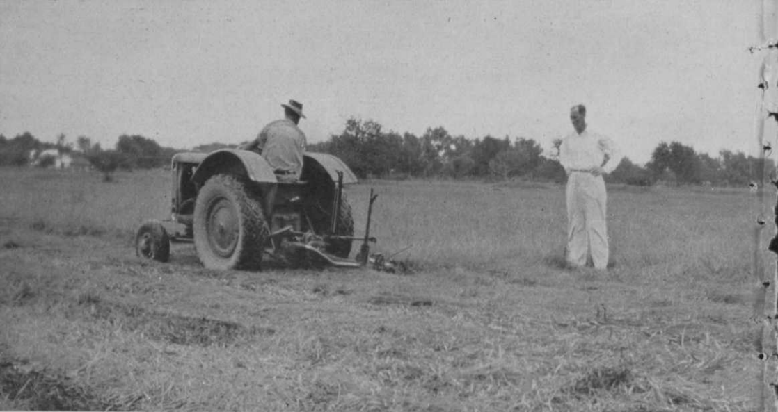
Fred Haas watching the International Fairway Tractor cut grass with a power mower which it operates through the power take-off.
