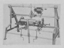
the sharpener, the makers claim, nor is it necessary to take the mower apart, since the whole unit is placed in the sharpener and the actual sharpening is almost automatic.
