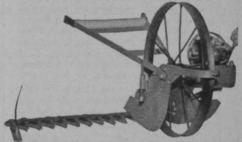
unit formerly used in this mower, when it was known as the Rawls motor scythe. This added power permits the sickle to saw through growths of weeds and brush that would stall a horse-drawn mower.
