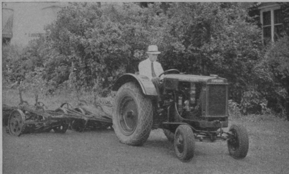
McCormick-Deering Fairway 12 Tractor equipped with low-pressure pneumatic tires which are available on special order. Steel wheels are furnished regularly.
