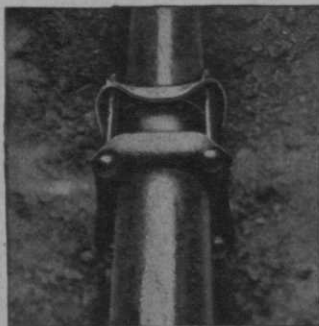
(Above) Note the adaptability of the flexible coupled line to the contour of the ground.
