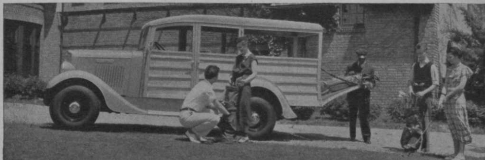
The new International Model C-1 Half-Ton chassis equipped with station-wagon body for passenger transportation combined with light loads.
