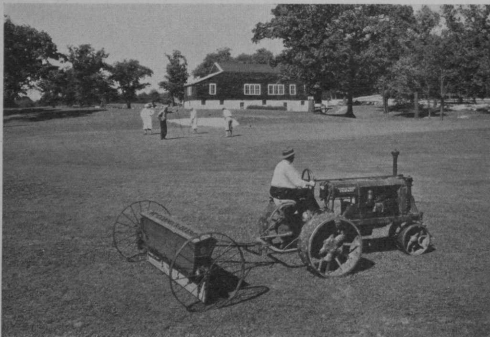
A McCormick-Deering Fairway Tractor and McCormick-Deering Fertilizer Distributor, with combination wind shield and scattering boards, building up a good turf on the fairways.
