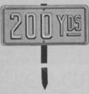
Plate-24 gauge galvannealed steel, guaranteed Rust Proof -Size 51/2x12-Finish highest grade flexible enamel, baked in two color contrasts.
