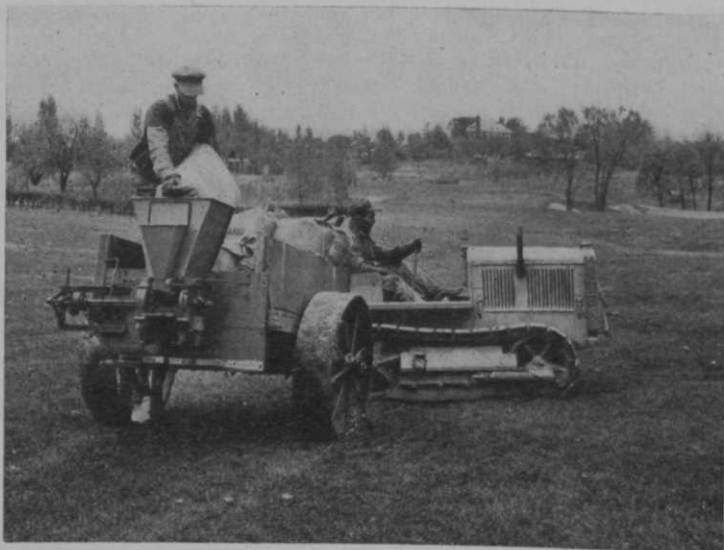
Fewer men, more machinery, the outstanding features of course maintenance in 1930, is exhibited at Peoria (Ill.) C. C. where a versatile Caterpillar tractor hauls a fertilizer-spreader as part of its work in contempt of traditional time-clock restrictions.
