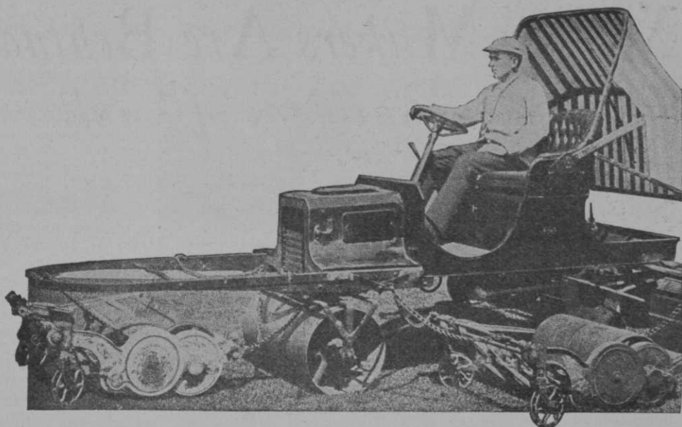
Home-made gang mower, with body and rear of a 1907 Reo runabout mounted on triple-armed frame. A 3-ft. mower was attached in front of the roller and another at the left side. It cut fairways of a Massachusetts club in 6-ft. swaths at a speed of 6 miles an hour. Pennsylvania Lawn Mower works furnishes this illustration by way of contrast with its modern equipment.
