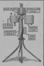
The Sure-Clean Washer will clean one to six balls at a time, and every mesh and dimple on the entire surface of the ball will be cleaned regardless of its condition.
