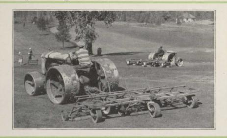
The low wheels on the Bulldog cutting unit permit a simple pinion-and-pawl drive. High wheeled mowers necessitate a chain-of-gears drive that can cost high when it goes wrong. Bulldog repairs can be made quickly, right on the job.
