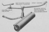
1.—The new Control Valve controls the speed of the Rotor and the quality of its spray under varying pressures. It eliminates those smoky sprays that are often lost in the breeze. It prevents excessive wear of the Rotor bearing.
