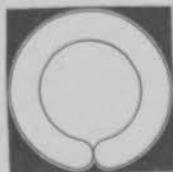
Cross-section showing improved torsion principle of construction—double walls, torsion seam.
