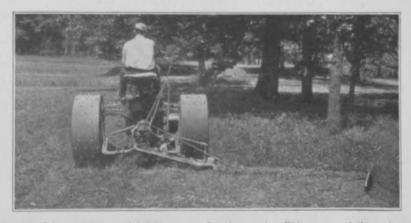
Showing the fairway with special 7-ft. mower for the rough. This tractor delivers its ample power three ways—through drawbar, belt, and power take-off. It is in itself a roller; wheels do not track, the weight being distributed to all 4 wheels. With gang mowers it cuts 75-100 acres a day. Pulls rollers, compost distributors, wagons. Ready for heavier jobs, plowing, disking, seeding, etc.; moves dirt, materials, and all equipment.
