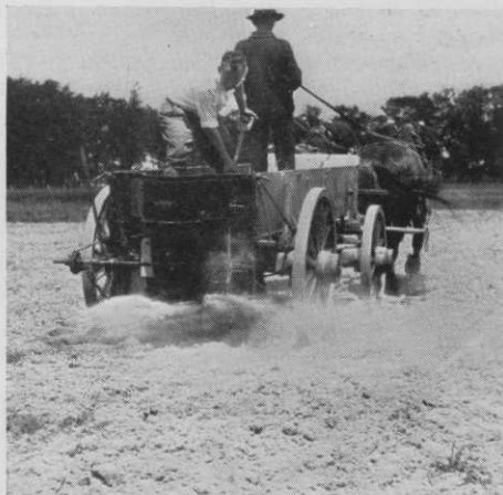
The endgate type spreader, attached to rear of wagon box. Fertilizer is fed into the hopper by shovel or poured from bags, and spreads by the machine in a fifteen-foot strip.
