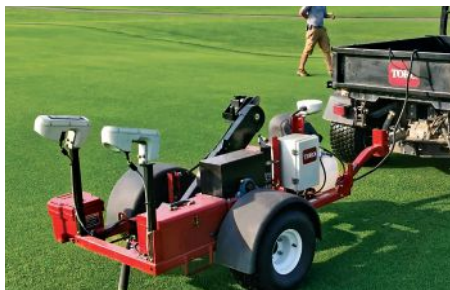
The Toro PrecisionSense provides an irrigation audit based on soil moisture, compaction, salinity, turf vigor, topography and slope.
