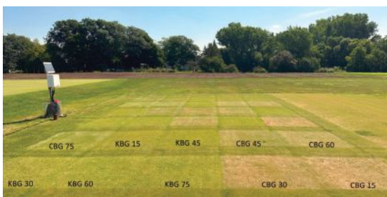
Creeping bentgrass and Kentucky bluegrass fairway turf plots were maintained at different soil moisture thresholds (15, 30, 45, 60 or 75 percent plant available water) on Aug. 3 at the University of Minnesota, St. Paul, Minn.
