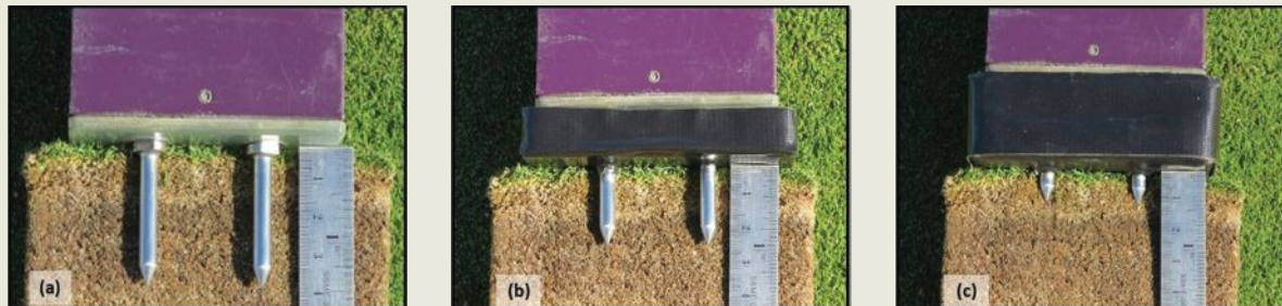
Field Scout TDR300 Soil Moisture Meter and (a) standard 1.5-inch turf rods. Researchers fit spacer blocks (black) onto 1.5-inch rods to achieve new measurement depths of (b) 1 inch and (c) 0.5 inches.
