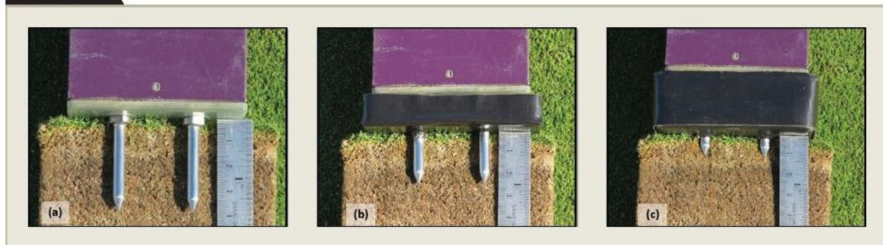
Field Scout TDR300 Soil Moisture Meter and (a) standard 1.5-inch turf rods. Researchers fit spacer blocks (black) onto 1.5-inch rods to achieve new measurement depths of (b) 1 inch and (c) 0.5 inches.
