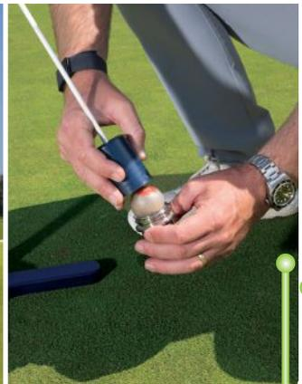
USGA's GS3 is a Bluetooth-enabled golf ball that measures speeds, firmness, trueness and smoothness. Measurements upload to USGA's Deacon app. Superintendents place the ball in a drop fixture to measure firmness.
