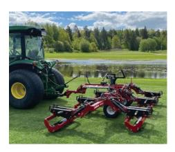
mower to their course to get the maximum mowing done in the shortest amount of time. Other innovative options include 100-hour greasing interval PTO shafts, Adaptive Swivel Hitch, HEX drive roller end and bearings — all time-saving elements to help reduce superintendents' mowing costs and prevent downtime.
