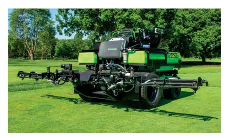
chemicals more efficient. The SGXL comes standard with a 2.5-gallon foam marker, which helps prevent overlapping or missing applications.
