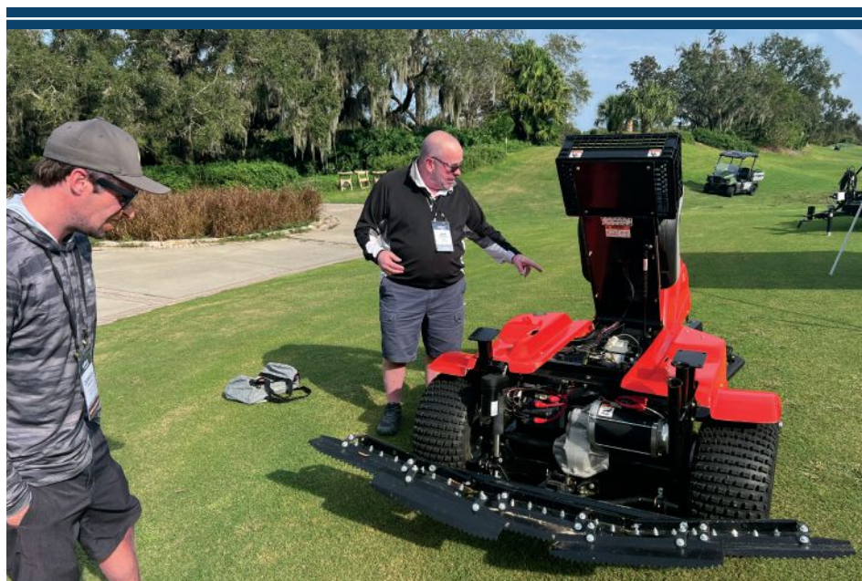
Jeff Churchill of Smithco walks superintendent Derrick Dreyer of Frost Creek through Smithco's battery-powered bunker rake.
