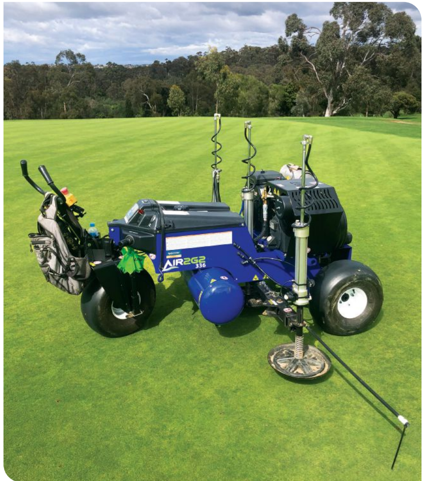
The Air2G2 336 uses three probes to laterally inject pressurized air up to 12 inches beneath the surface of the soil, in a diameter of up to 9 feet, reaching deep into the soil profile.
