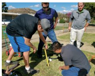
Students install a Rain Bird Integrated soil moisture sensor in the bermudagrass fairway plot
