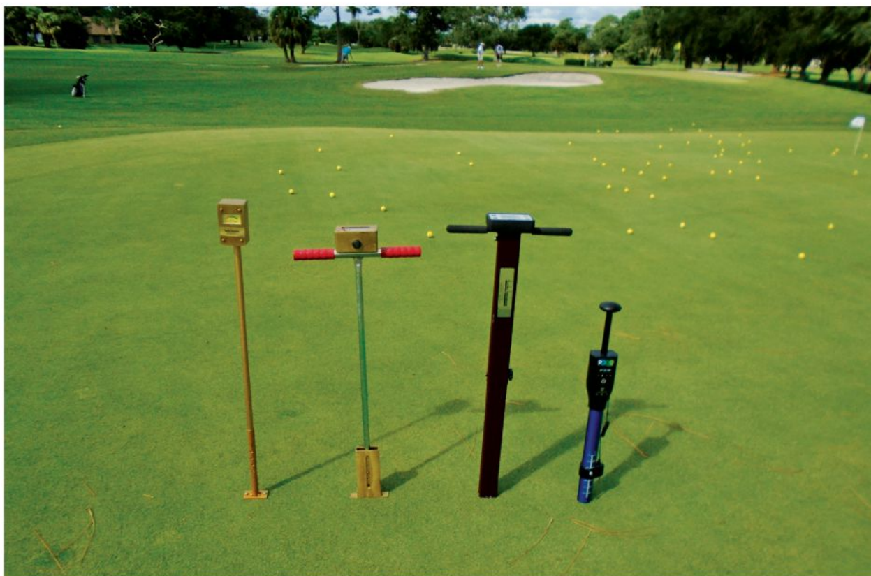
Soil moisture sensors such as the Turf-Tec, Field Scout and Pogo models pictured reduce the risk of overwatering greens.
