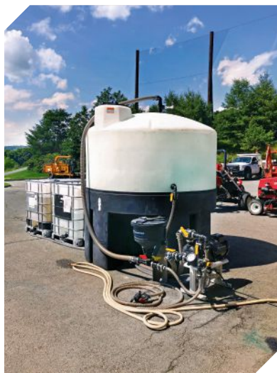
Kraft uses a 1,600-gallon mix tank from SynaTek, saving two hours of spray time.
