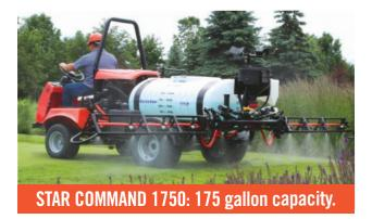
35 hp (23 kW) air-cooled, twin-cylinder gas engine. TeeJet Aeros GPS Satellite provides Sub - 5 CM position control and permanently retained mapping. Smithco/TeeJet DynaJet Pulse Width Modulation (PWM) allows you to spray from 2 to 10 MPH without changing droplet size.
