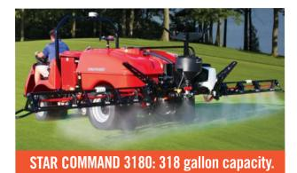
Compact, maneuverable, large-capacity sprayer, powered by a 49 hp 4-cylinder liquid cooled gas engine. TeeJet Aeros GPS Computer provides Sub - 5 CM position control. Smithco/ TeeJet DynaJet Pulse Width Modulation (PWM) allows you to spray from 2 to 10 MPH without changing droplet size.
