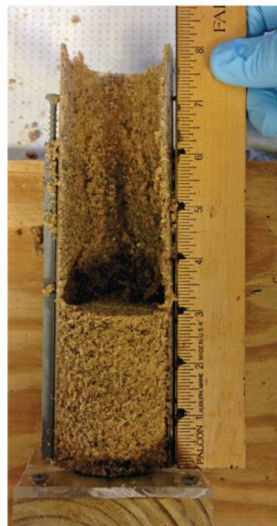
Sectioning soil into 1-inch increments to recover applied ^{14}\text{C} -fungicide.
