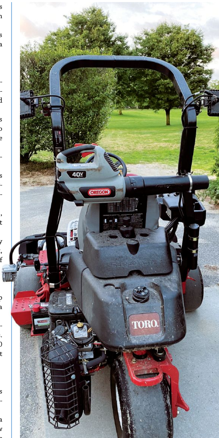
These greens mowers tackle North Hempstead CC's 22 greens with handheld blowers and backup batteries.
