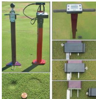
Measurement devices used in this research. From left to right: TruFirm, Clegg and TDR350 with Turf Rod Spacers at 0.5-, 1.0- and 1.5-inch depths.
