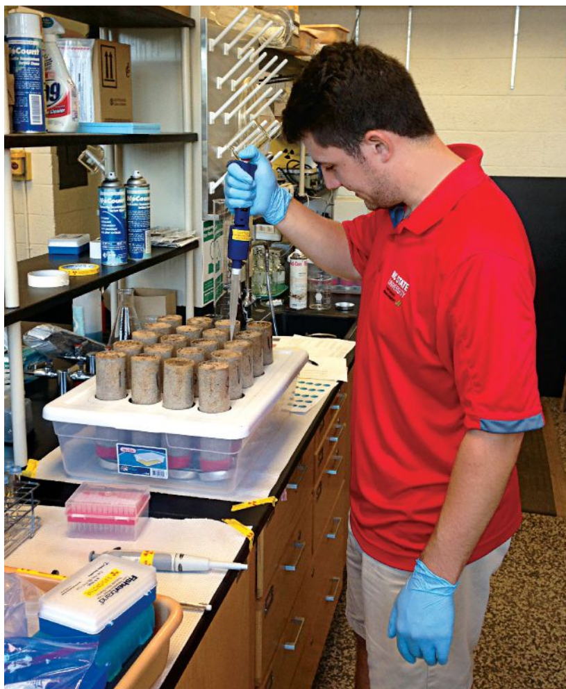
Application of post-application irrigation with a pipette to soil contained in lysimeters.
